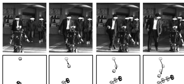
Fig. 1 The video frames and the illustrations show a real world situation in which using a traditional collision-avoidance method generated a possibly unsafe situation. (a) Initially, the pedestrian did not notice the robot. (b) Then he unexpectedly found the robot in front of him and felt unsafe although the robot had already started to avoid him; (c) as a consequence the pedestrian quickly moved aside and (d) looked at the robot with surprise.
